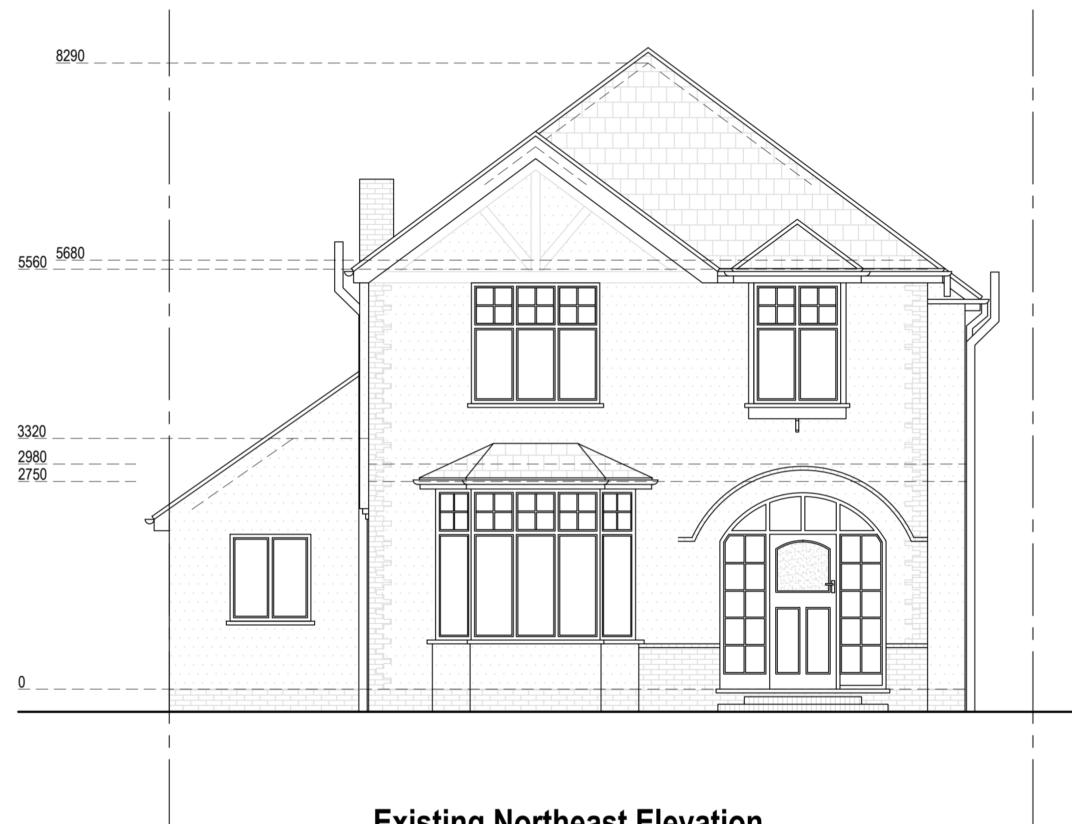
Existing Northeast Elevation Scale 1:50
